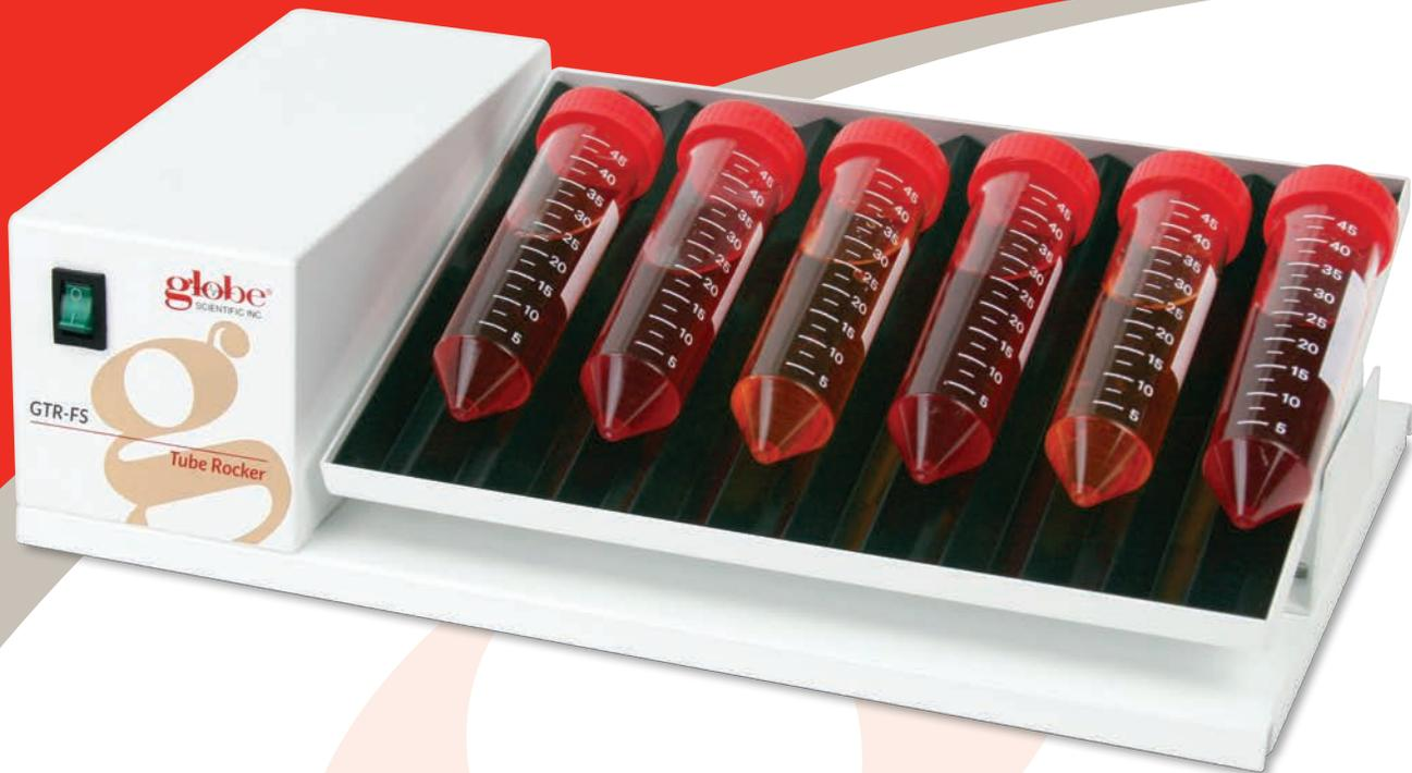
The GTR-FS fixed-speed tube rocker is the best choice for basic laboratory tube mixing applications. With its see-saw motion, a fixed speed of 24rpm and an angle of +/-25° it provides optimal mixing. The ridged platform pad design allows the operator to place any tube from 1.5mL to 50mL on the unit, turn the power switch on and walk away.
